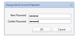
The only other way of changing the serial console password is in the *boot menu* which can be entered from the serial console during startup. The InControl option offers a way to change the password without disruption to traffic.
