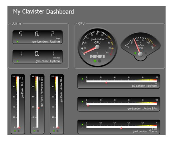
The image above illustrates a dashboard consisting of *Gauge* monitoring controls in various styles. Each Gauge is monitoring a single parameter in a cOS Core installation.
